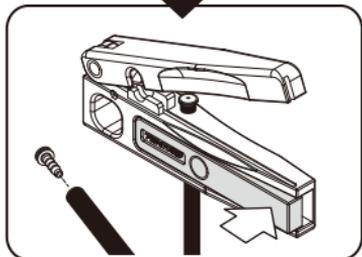
Put compression insert with O-ring into the tubing. Put tubing through the hole at the bottom of base and press the clip to hold the tube.
