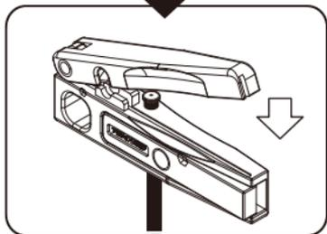
Push down the cutter to press insert into tubing properly.
