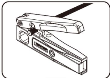
Put tubing in the cutting groove and pushed down the cutter to cut the required length. Tubing must to be flat and free of burrs.
